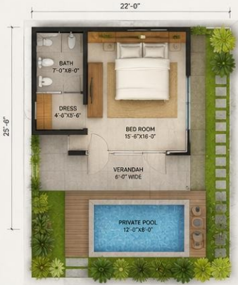
FLOOR PLAN (Total Built-up Area: 560 sft)
